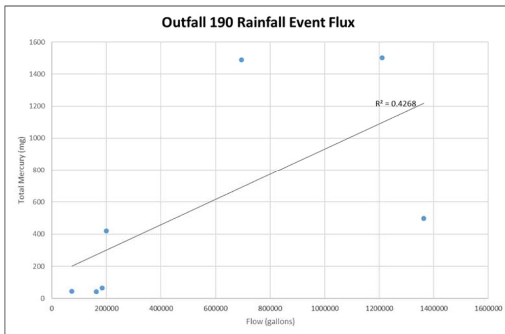
**Figure 3.17. Flow-proportional mercury sampling at Outfall 190**
