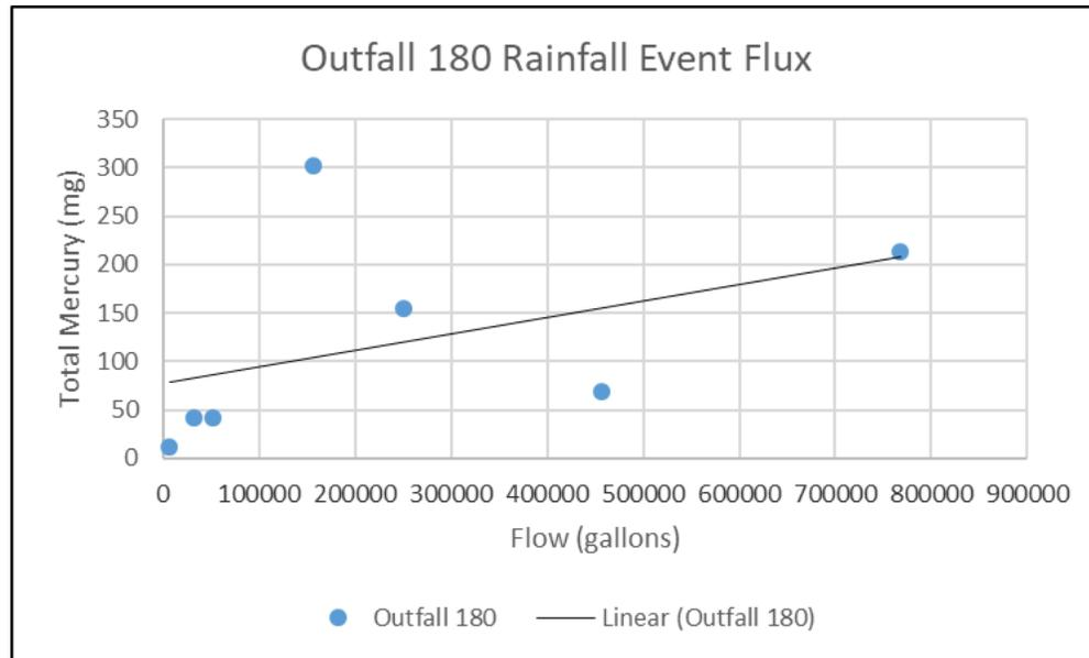
Figure 3.15. Flow-proportional mercury sampling at Outfall 180
